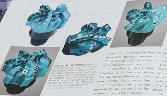
**THE TIP OF THE SPEAR:** Ultrerra manufactures a wide variety of drill bits as its factories in the U.S. and Canada. From the top left clockwise: a FastBack bit for enhanced rate of penetration, a CounterForce bit for vibration control, a bit developed for drilling in China, and a SplitBlade bit for improved cuttings evacuation.
